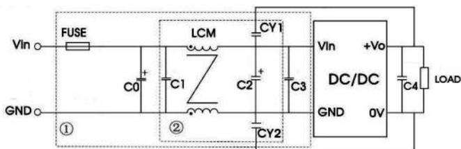
Notes: For EMC tests we use Part ① in Fig. 3 for immunity and part ② for emissions test. Selecting based on needs.
