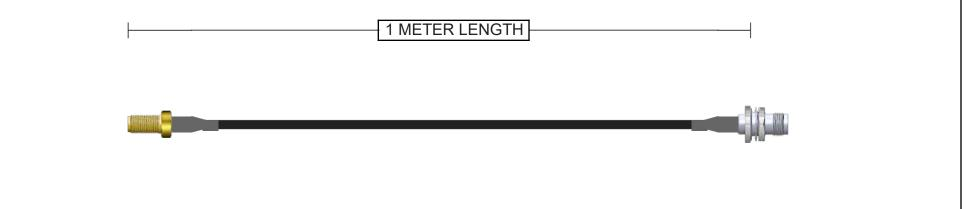
Connector A 132117 SMA Jack Straight Brass Gold + Heatshrink 50 Ohm RG-174 Continuity/Hi-Pot Connector B 122192-15 TNC Jack Straight Bulkhead - Rear Mount Brass Nickel IP67 + Heatshrink
