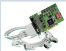
UC-368: uPCI 4xRS422/485 1MBaud Opto Isolated
