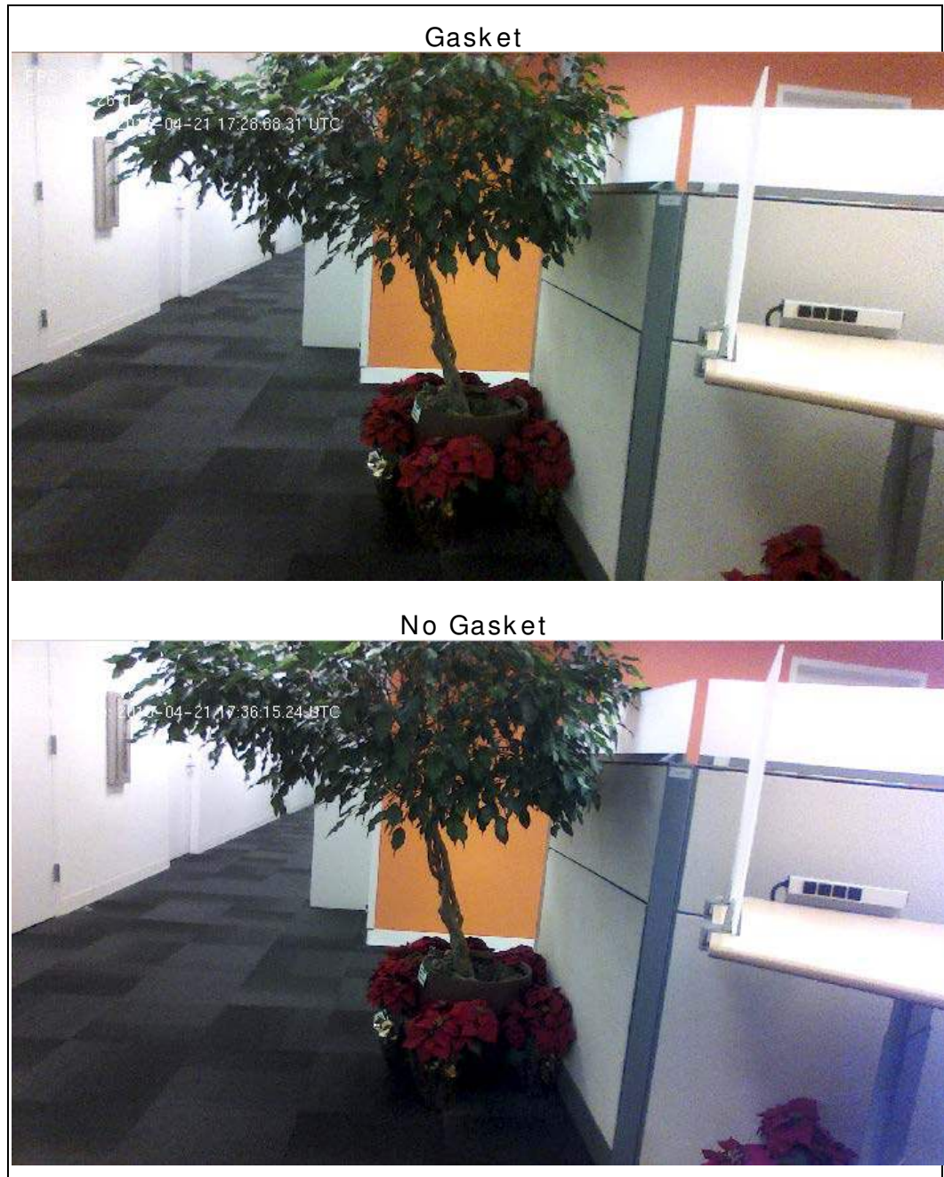
Figure 7-6. Example of Light Leakage Effects
