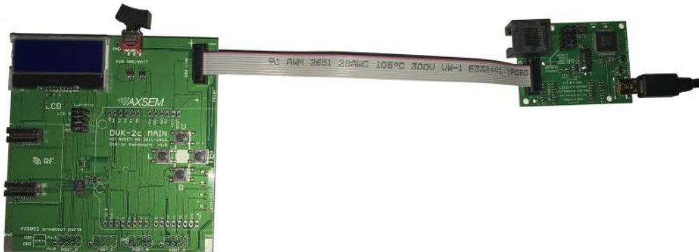
Figure 3. DVK-2 Main Board Connected to the AXDBG
