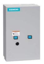
2-speed 3-phase motor starter, Size 0, Two separate windings, Constant or variable torque, Solid-state overload relays, Low Spd OLR range 0.75-3.4A, High Spd OLR range 3-12A, 110V 50Hz / 120V 60Hz coil, Enclosure NEMA type 1, Indoor general purpose use
