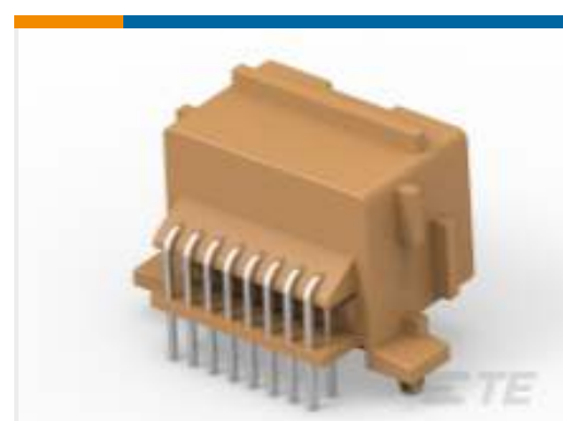
TE Part #966870-2 16POS,TAB0.63X0.63,HDR ASSY,90 DEG,COD A
