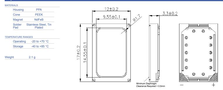
General tolerance =  $\pm 0.2$  mm and all measurements in mm unless otherwise noted.
