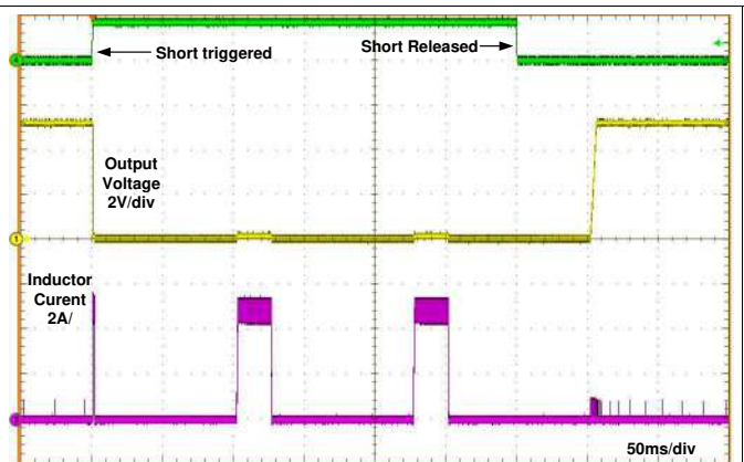
Figure 6. LM60440 Short-Circuit Transient and Recovery
