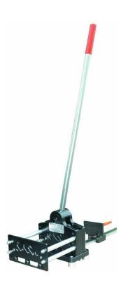
The TS-PSS 2 DIN rail cutter and punching tool is designed for manually shortening and punching holes in DIN rails (TS 15, TS 35, TS 32) and busbars ( $10 \times 3 \text{ mm}$ ). The tool can be mounted on a workbench or similar working surface. It can also punch holes of varying dimensions in customized positions. A cross-hole/slotted-hole punch ( $12 \times 6.4 \text{ mm}$ ) is included in the delivery.
