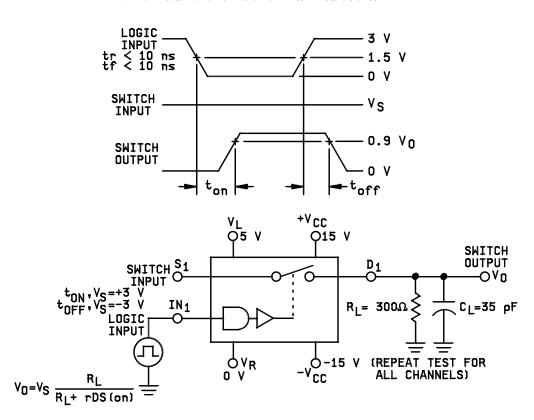
$V_O$  is the steady state output with the switch on. Feedthrough via switch capacitance may result in spikes at the leading and trailing edge of the output waveform. Switch output waveform shown for  $V_S$  = constant with logic input waveform as shown. Note that  $V_S$  may be + or – as per switching time test circuit.
