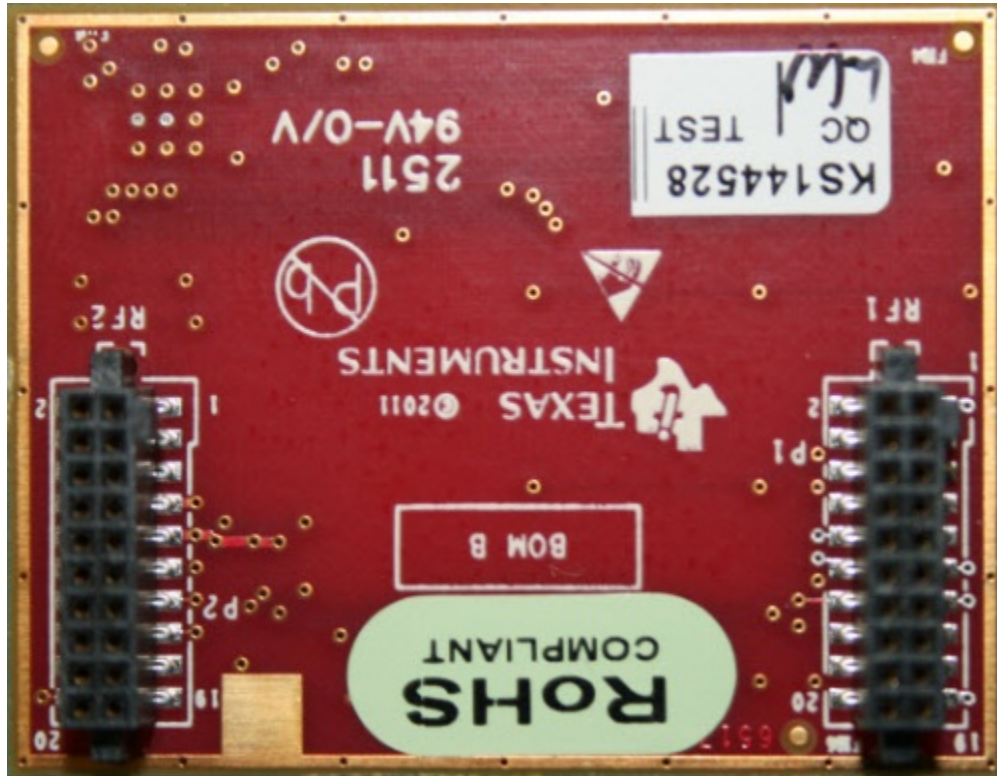
Figure 6. Back side of the RF-TCA8418-MVK MAVRK Module, showing the RF connectors
