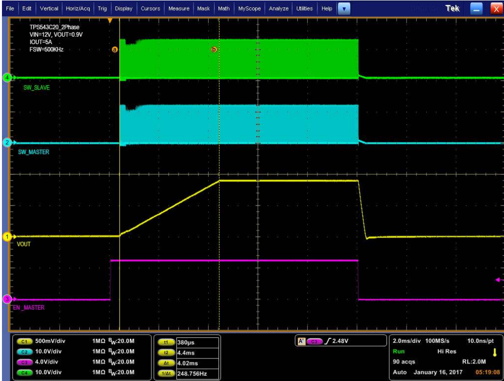
Figure 9-11. Output Voltage Start-Up and Shutdown, 0.9-V Output at 12 V IN , 5-A Output
