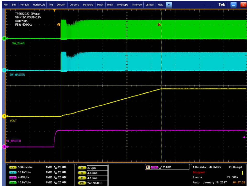
Figure 9-9. Start-Up from Enable, 0.9-V Output at 12 V IN , 80-A Output
