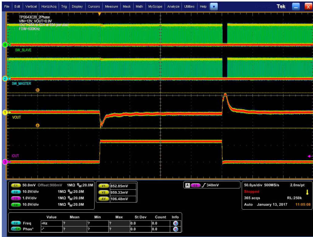
Figure 9-4. Transient Response of 0.9-V Output at 12 V IN , Transient is 25 A to 50 A, Step is 25 A at 30 A/μs
