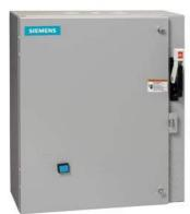
Non-reversing motor starter, Size 3, Three phase full voltage, Solid-state overload relay, OLR amp range 25-100A, 24VDC coil, Combination type, 100A fusible disconnect, 100A/250V fuse clip, Enclosure NEMA type 1, Indoor general purpose use, Standard width enclosure
