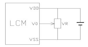
V<sub>DD~</sub>V<sub>0</sub>: LCD Driving voltage VR: 10k~20k
