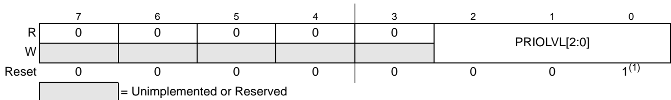
Figure 4-12. Interrupt Request Configuration Data Register 7 (INT_CFDATA7)
