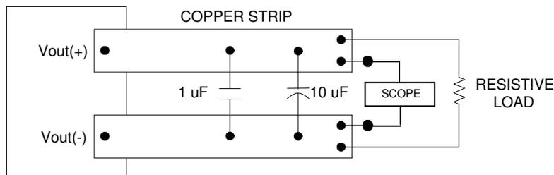
Note: Use a 1 $\mu\text{F}$  X7R ceramic capacitor and a 10 $\mu\text{F}$  tantalum capacitor. Scope measurement should be made using a BNC socket. Position the load 3 in. [76mm] from module.
