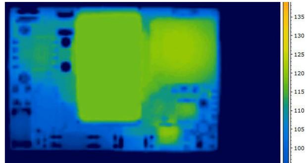
Figure 4. Thermal Image of CPT3L48 3A output, 85C Ambient, 200lfm airflow, Vin = 48V, airflow from pin 3 to pin 1, T<sub>max</sub> = 119°C
