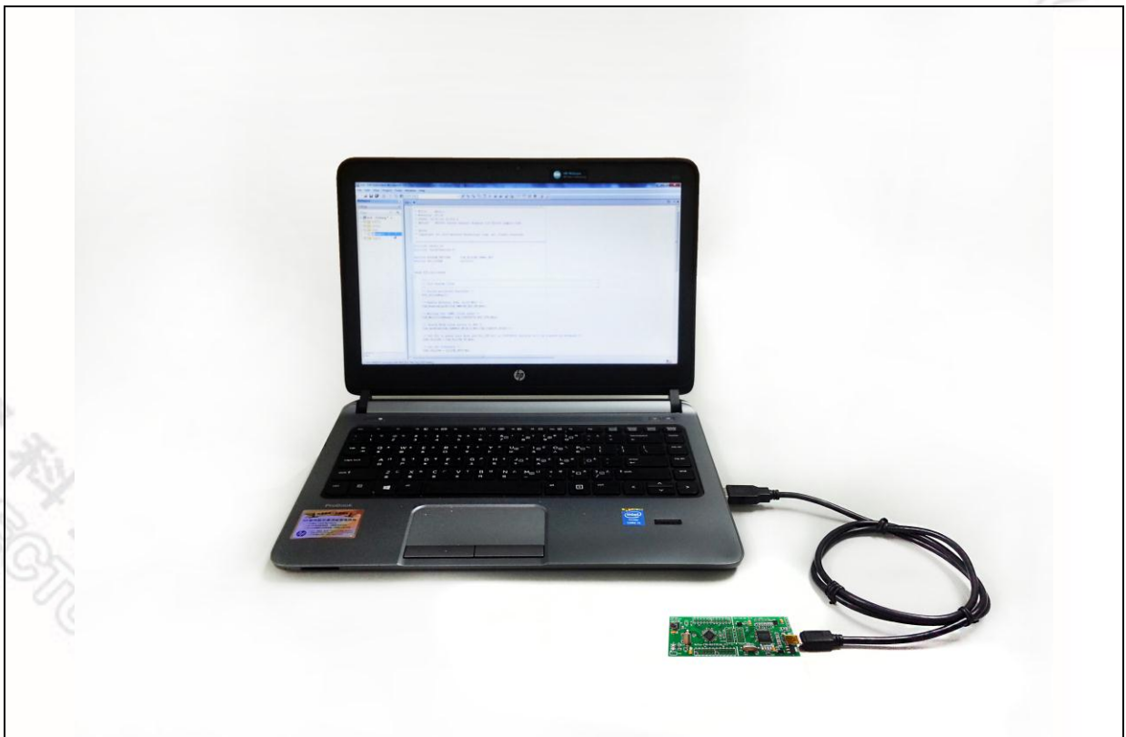
Figure 4-1 NuTiny-SDK-NUC029LAN Hardware Setup
