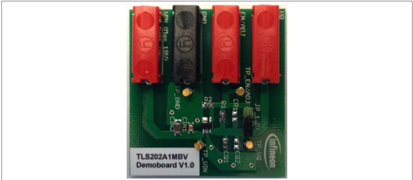
Figure 2 TLS202A1 Demo Board
