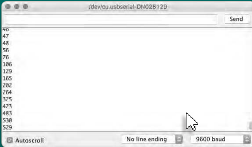
Serial Monitor printout and baud-rate menu.
