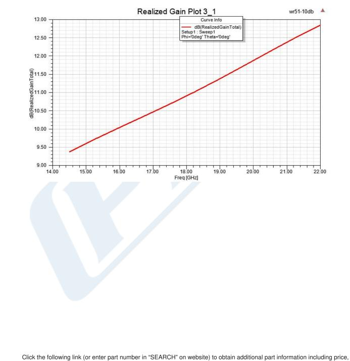
inventory and certifications: WR-51 Standard Gain Horn Antenna Operating From 15 GHz to 22 GHz, 10 dBi Nominal Gain, square Flange PEWAN051-10
