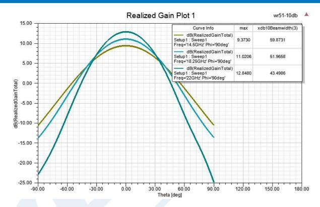
WR-51 Standard Gain Horn Antenna Operating From 15 GHz to 22 GHz, 10 dBi Nominal Gain, square Flange from Pasternack Enterprises has same day shipment for domestic and International orders. Our RF, microwave and millimeter wave products maintain a 99.4% availability and are part of the broadest selection in the industry.
