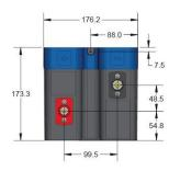
Positive Terminal: 5/16" – 18 threaded stud Negative Terminal: 3/8" – 16 threaded stud
