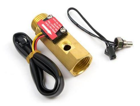
It consists of a copper body, a water rotor, and a hall-effect sensor. When water flows through the rotor, rotor rolls. Its speed changes with different rate of flow. The hall-effect sensor outputs the corresponding pulse signal.
