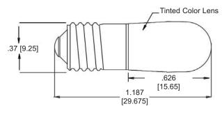
Measurements are typical Dimensions are inches [mm]
