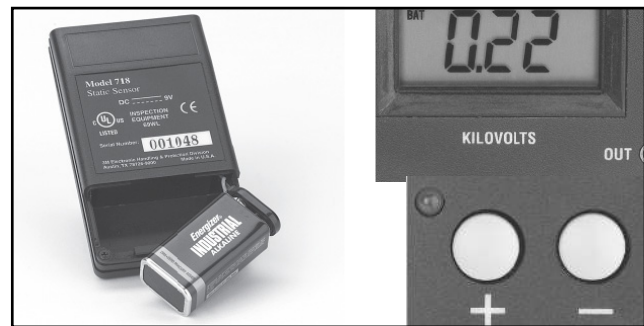
Figure 2. SCS 718 and 718A Battery Replacement and Indicators.
