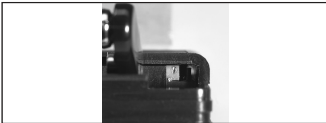
Figure 9. 718 Static Sensor adjustable screw for display.
