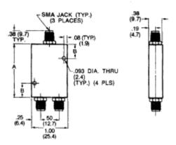
Note: All dimensions are  $\pm$  .020, except mounting hole diameters ( $\pm$  .005) and mounting hole location ( $\pm$  .010) .
