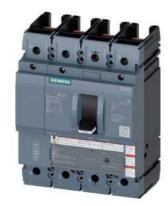
circuit breaker 3VA5 UL frame 250 breaking capacity class H 65kA @ 480V 4-pole, line protection TM230, FTAM, In=80A overload protection Ir=80A fixed short-circuit protection Ii=5...10 x In N conductor unprotected without connection
