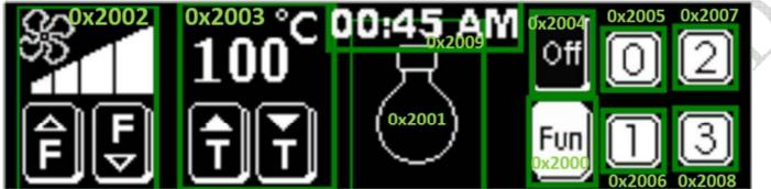
0x2000 Toggle Button 0x2001 Animated Image 0x2002 Custom Widget 0x2003 Custom Widget 0x2004 Toggle Button 0x2005 Toggle Button 0x2006 Toggle Button 0x2007 Toggle Button 0x2008 Toggle Button 0x2009 Digital clock
