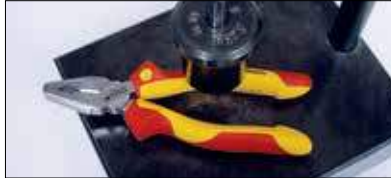
Cold Impact Test
