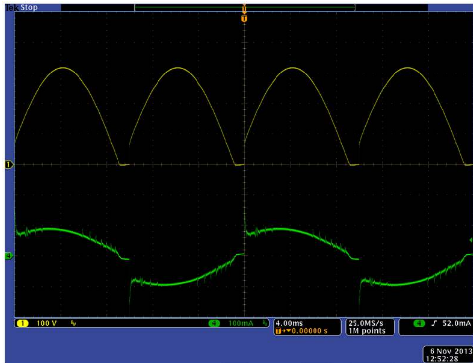
Figure 6. Forward Phase Triac Dimming: Rectified Input Voltage (Top) and Input Current (Bottom)
