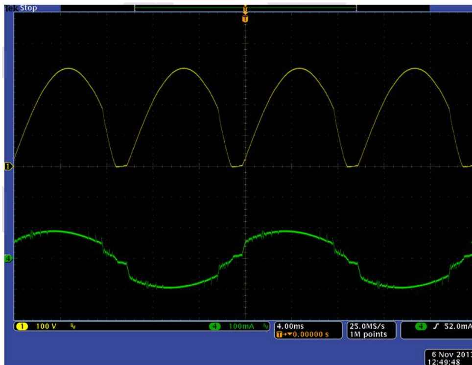
Figure 9. Reverse Phase Triac Dimming: Rectified Input Voltage (Top) and Input Current (Bottom)
