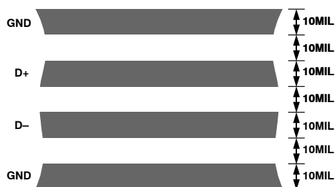
Figure 34. Arrangement of Signal Tracks
