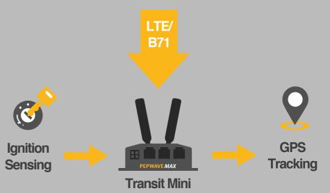
The MAX Transit Mini provides cellular connectivity for passengers. It connects using LTE, supporting band 71 for improved range and signal penetration. This means the Transit Mini will stay connected even in remote areas where other bands drop off.
