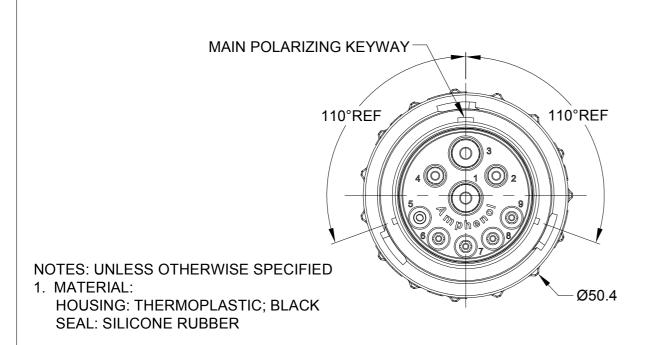
REV ECO **DESCRIPTION** DATE **APPR** 38.5 RELEASE NEW DRAWING 13NOV20 IAN A1 TOMMY 10.7 SIZE 12 CONTACT (2 PLACES) /8` SIZE 8 CONTACT (2 PLACES) Ø40.4 SIZE 16 CONTACT (5 PLACES) **SEALING PLUG** 1 11/16-12 UN -2A 5 6 **THREAD**
