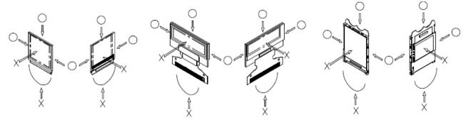
7) Do not apply stress to the driver IC and the surrounding molded sections.
