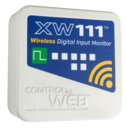
The XW-111 is an easy-to-use, wireless digital input monitoring device with a built-in web server. The XW-111 monitors and reports the status of switch closure sensors and alarms. It's ideal for applications where a device's status must be monitored and Ethernet wiring is not accessible or practical to install.
