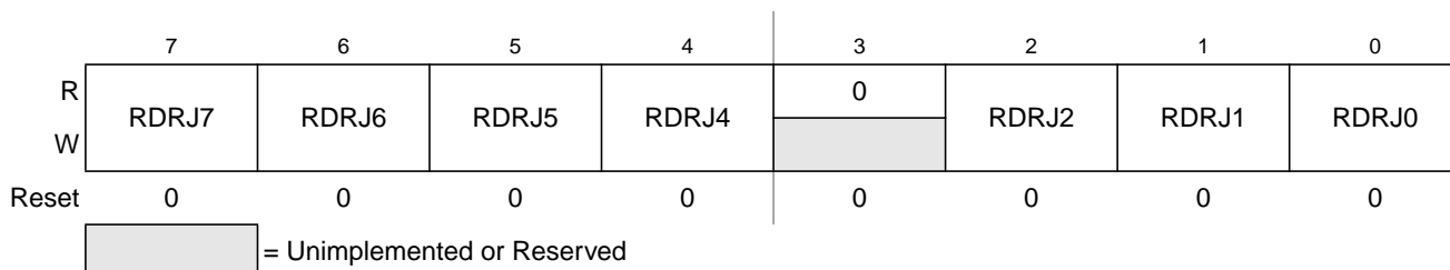
Figure 23-59. Port J Reduced Drive Register (RDRJ)
