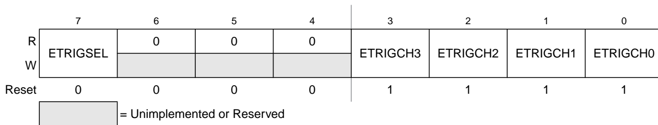
Figure 4-4. ATD Control Register 1 (ATDCTL1)
