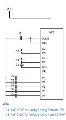
*NOTE:* See IC controller spec NT7534 for more information on internal voltage regulating circuits. Additional information on DC-DC voltage regulating circuits for graphic LCD's is available on our website at <u>www.FocusLCDs.com.</u>
