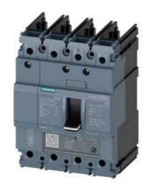
circuit breaker 3VA5 UL frame 125 breaking capacity class H 65kA @ 480V 4-pole, line protection TM230, FTAM, In=110A overload protection Ir=110A fixed short-circuit protection Ii=5...10 x In N conductor unprotected without connection
