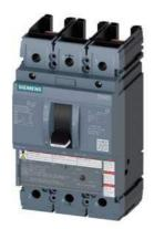
circuit breaker 3VA5 UL frame 250 breaking capacity class C 100kA @ 480V 2-pole, line protection TM230, FTAM, In=100A overload protection Ir=100A fixed short-circuit protection Ii=5...10 x In without connection
