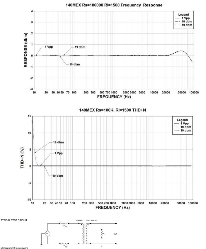
Measurement instruments Hp4192a impedance analyzer Hp3456a DVM Keithley 2002 DVM D scope series iii audio analyzer
