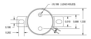
This transformer operates in the 20 Hz to 20 KHz range. The metal can provides excellent shielding from a broad range of external sources. The nickel core provides high permeability combined with low losses.
