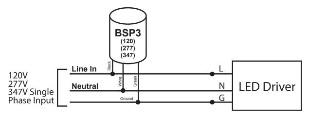
BSP3 and driver voltage must match input voltage
