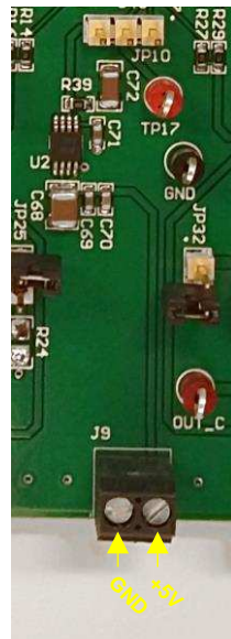
Figure 5. Onboard Reference Supply Connections
