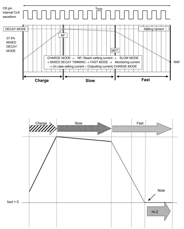
Note: When the motor current reaches zero level (Iout = 0 A), the output becomes "Hi-Z" state.
