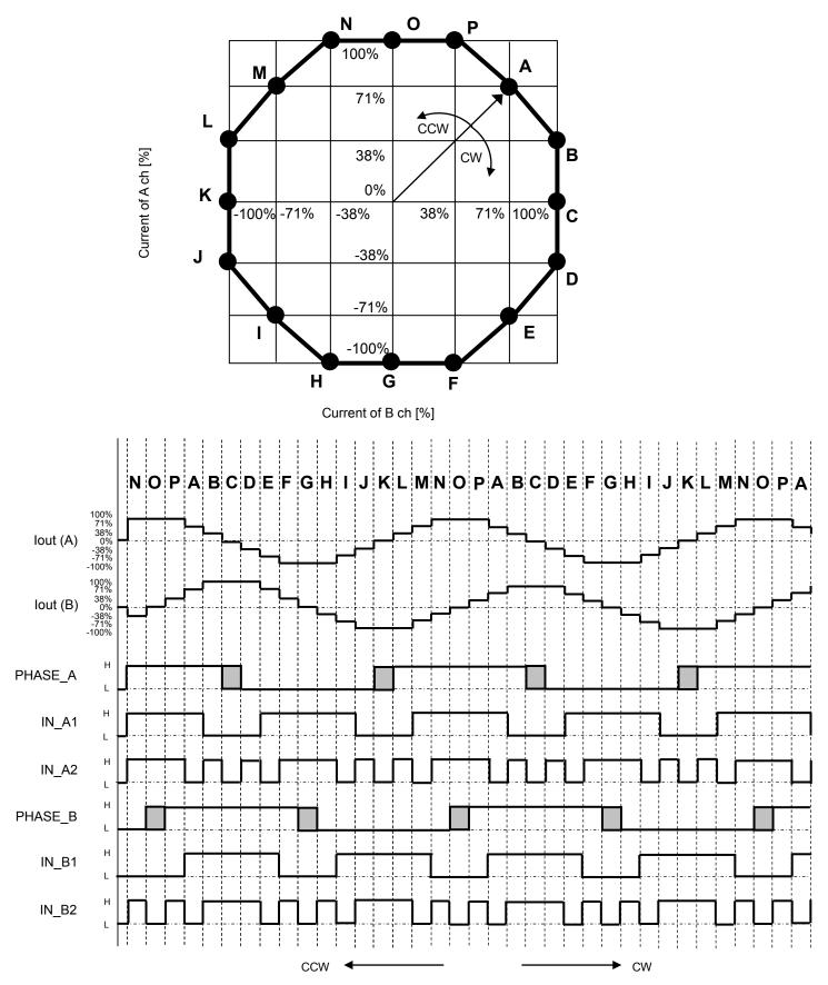
Timing charts may be simplified for explanatory purpose. Please set IN\_A1, IN\_A2, IN\_B1, and IN\_B2 low in supplying a power.
