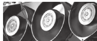
Fans in an endurance test cabinet at ebm-papst St. Georgen. 1500 fans are operated in temperature cabinets until they fail.
