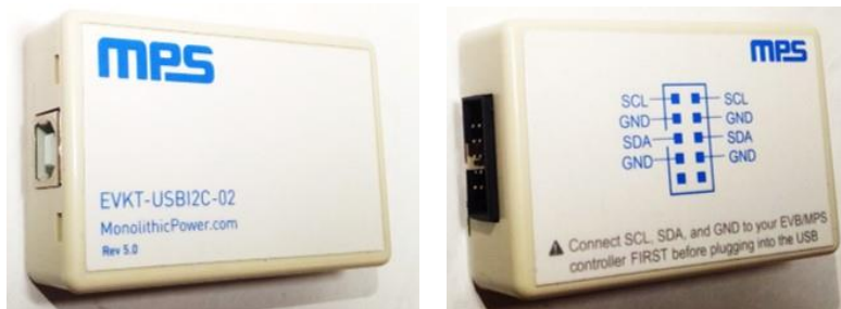
Figure 3: EVKT-USBI2C-02 Communication Interface
