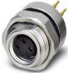
Sensor/actuator flush-type connector, female, 3-pos., M8, rear/screw mounting with M12 thread, with straight solder connection
