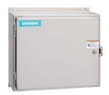
Mechanically held lighting contactor, Contactor amp rating 60Amp 0NC  $\_$  6NO poles, 277VAC 60HZ coil, Non-combination type, Enclosure NEMA type 12, Dust/drip proof for indoors
