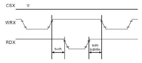
Note: Logic high and low levels are specified as 30% and 70% of IOVCC for Input signals.
