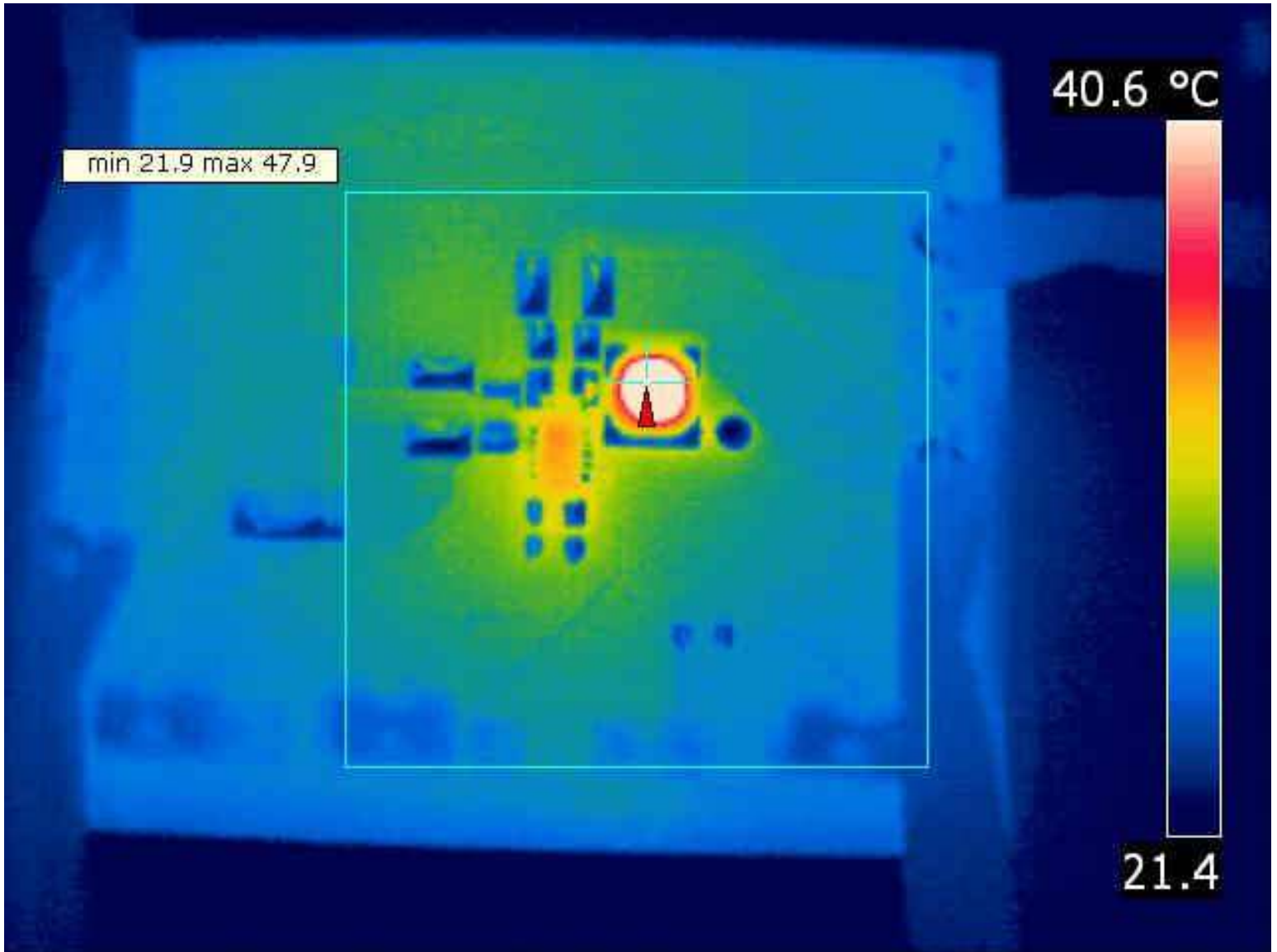
Figure 3-1. Thermal Performance ( V_{IN} = 12\text{ V} , Load = 500 mA)
