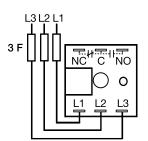
L1 = Phase A L2 = Phase B L3 = Phase C NO = Normally Open NC = Normally Closed C = Common, Transfer Contact
